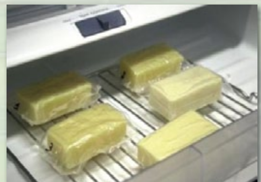
Researchers tested their milk-protein film as a packaging for blocks of cheese.
